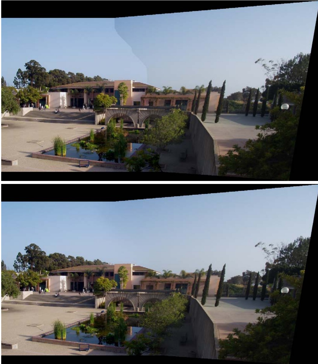
Figure 6.19: The equalization procedure described in Section 6.2.2 is not able to compensate for the photometric distortion and the seam between the images is very evident (top image). However the blending procedure is able to produce a seamless mosaic of the two images (bottom image).
