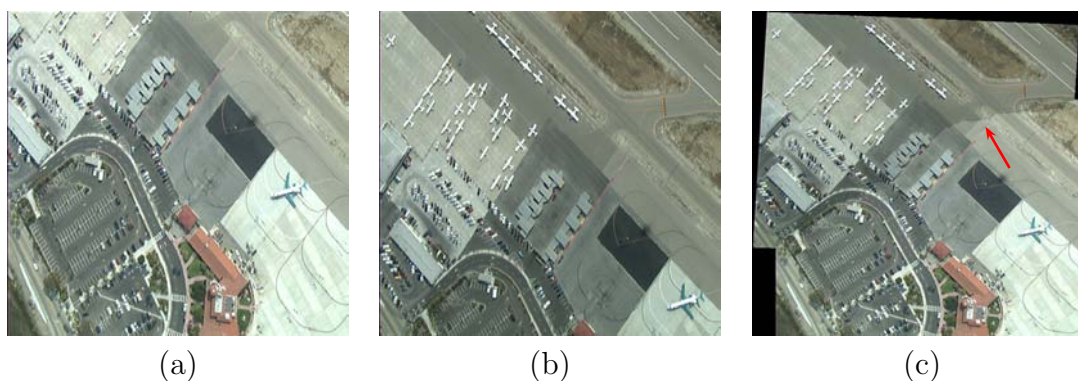
Figure 6.12: Images (a) and (b) show a pair of images to be mosaicked that are non equalized. The resulting mosaic is shown in image (c). The red arrow shows a detail near the stitching line where the different photometric properties of the images become very evident.
