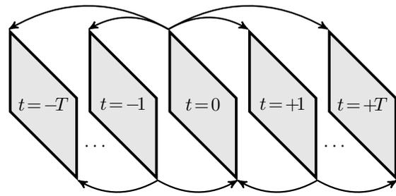
Figure 7. Pairs of frames considered for feature extraction. Ideally, there are  $4T^2 + 2T$  possible pairs. Although, practically, some of the pairs can be pruned to reduce complexity.
