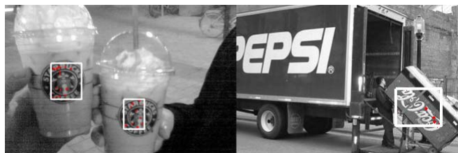
Fig. 1. Logo detection by clustering matching frequent spatial configurations of local features found by data mining.
