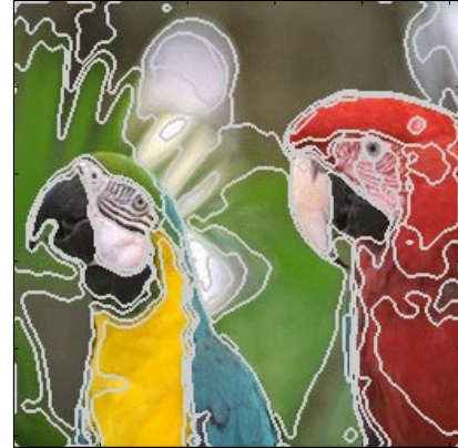
Figure 4. Original color images of Fig. 1 with borderlines drawn between homogeneous regions (there are C'' = 14 segments in both examples).
