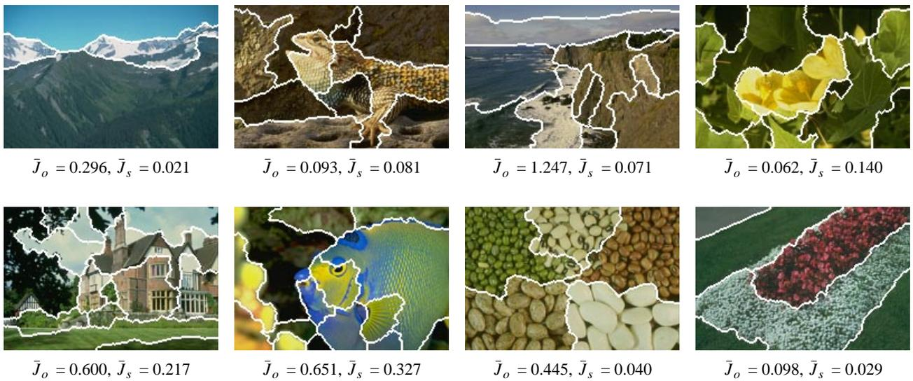
Fig 7. Example segmentation results on images from Corel photo CDs. 2,500 images are automatically processed without any parameter tuning on individual images. 1 scale, size 192 x 128,  $\bar{J}_o$  is  $\bar{J}$  calculated for the original image and  $\bar{J}_s$  is for the segmented one.
