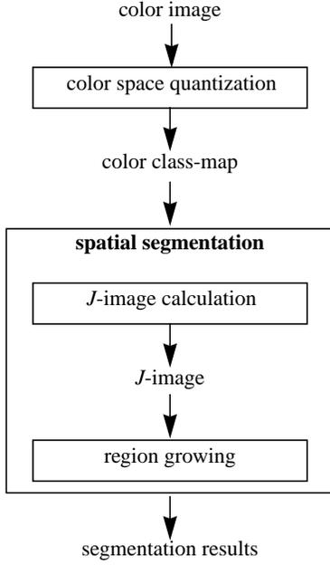
Fig 1. Schematic of the JSEG algorithm.
