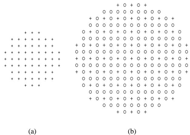
Fig 4. (a) the basic window for calculating local  $J$  values. (b) illustration of downsampling for the window at scale 2. Only ‘+’ points are used for calculating local  $J$  values, which forms the same basic window as in (a).
