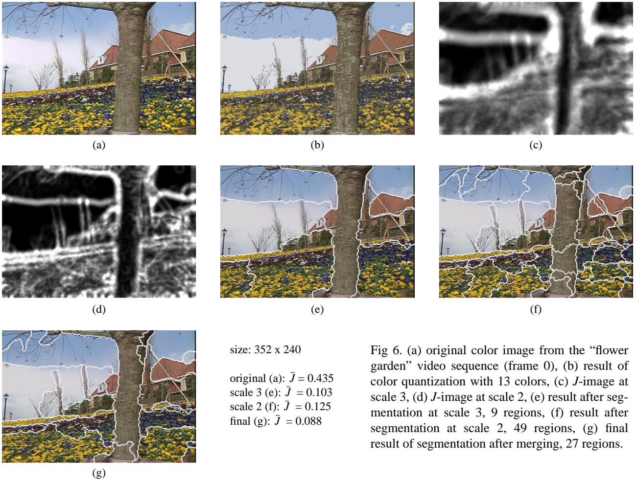
Fig 6. (a) original color image from the “flower garden” video sequence (frame 0), (b) result of color quantization with 13 colors, (c)  $J$ -image at scale 3, (d)  $J$ -image at scale 2, (e) result after segmentation at scale 3, 9 regions, (f) result after segmentation at scale 2, 49 regions, (g) final result of segmentation after merging, 27 regions.
