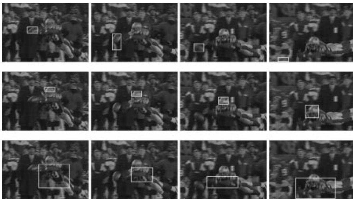
Fig. 10. Three identified subobjects in the same video sequence. The same consecutive I -frames are shown in each row. The three subobjects are, from top to bottom, a football, a player's head, and his upper body, respectively.
