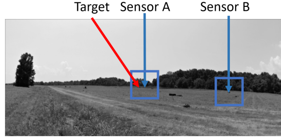
Figure 2. ROIs seen from a wider camera view. Each ROI is located around the sensor locations which are known a priori. Notice that in the figure, target is within the Sensor A’s region which produces a positive sample whereas the sample from Sensor B is a negative sample. There are multiple ROIs within this camera frame but only two of them are shown.
