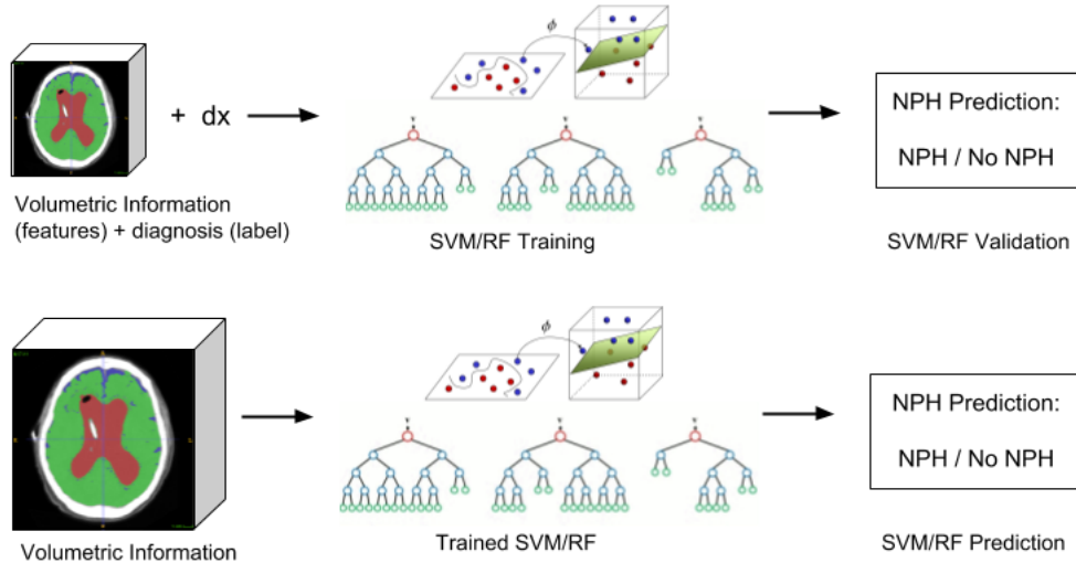
Fig. 6: Procedure for NPH prediction. The first row depicts the training stage and the second row depicts the prediction stage.
