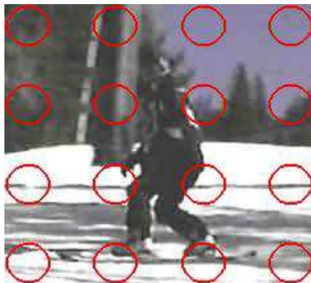
Figure 6.6: Initialization of the curve evolution for image segmentation.
