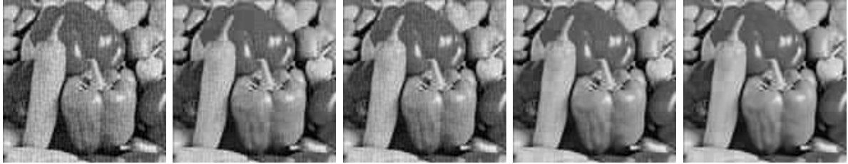
(a) attk. QF = 25 (93.5% compr.), MSE = 0.0286 (b) attk. QF = 45 (88.7% compr.), MSE = 0.0193 (c) attk. QF = 65 (85.0% compr.), MSE = 0.0119 (d) attk. QF = 85 (75.8% compr.), MSE = 0.0043 (e) No attack
