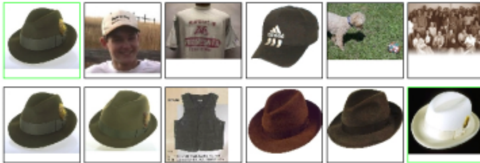
Figure 4 – Results of a constrained content-based search using the image selected in Figure 3. Top row shows query image and 5 most similar images with respect to the color descriptor. Bottom row shows query image and 5 most similar images with respect to the texture descriptor. The bottom right image is added to the query.
