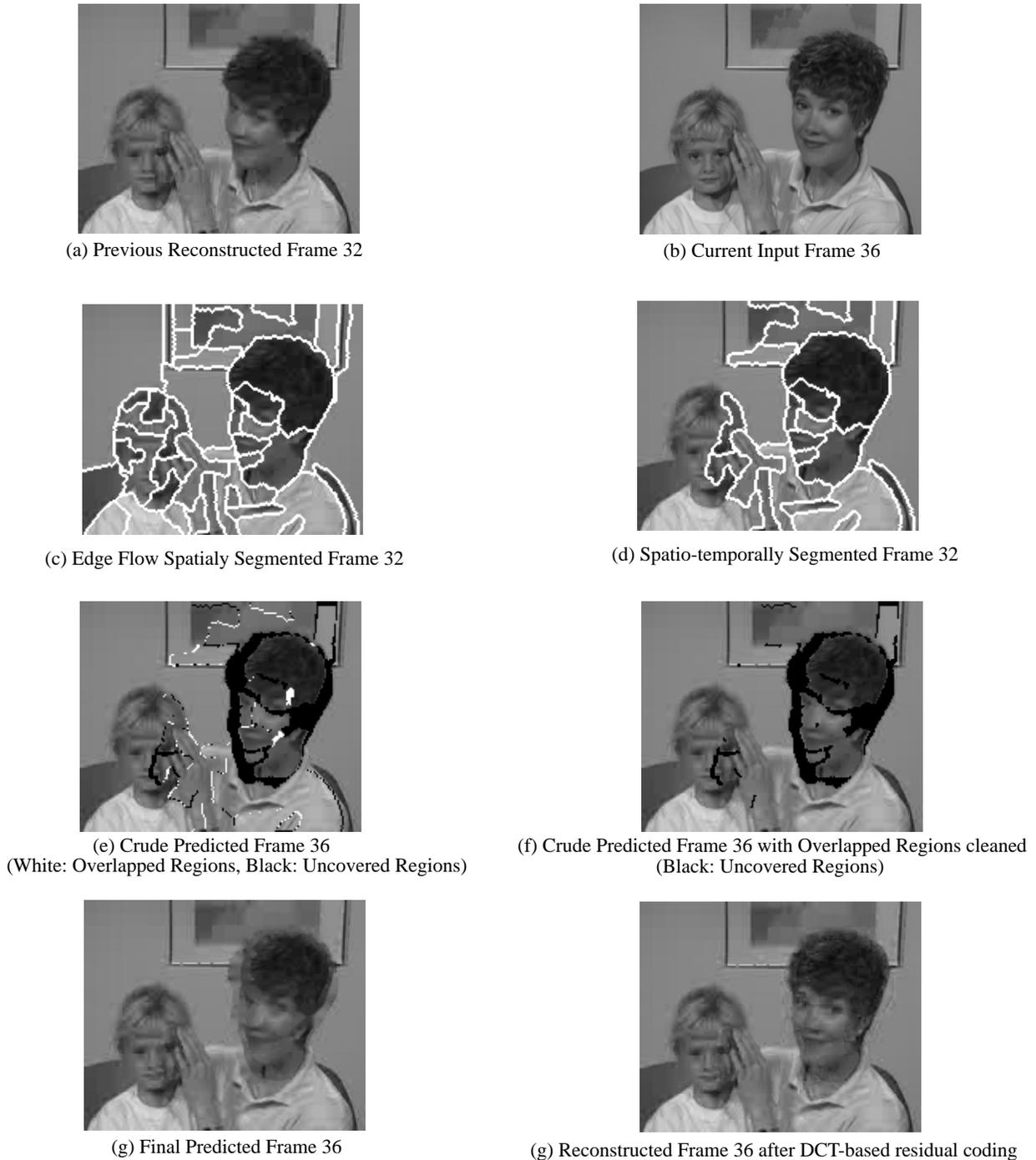
Figure 3. Illustration of the coding algorithm. Frame 36 of the mother-daughter sequence is coded from reconstructed Frame 32 at the frame rate of 7.5 frames/s.
