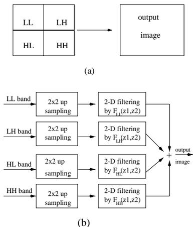
Figure 1: Two equivalent synthesis structures: (a) one level of synthesis; (b) the parallel implementation by 2-D filtering.
