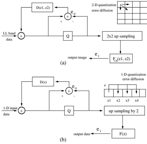
Figure 2: (a) the 2-D quantization error feedback structure. (b) the 1-D quantization error feedback structure.
