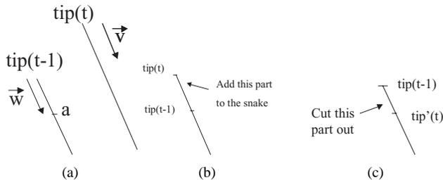
**Fig. 1.** (a) Illustration of the test performed to check if the curvilinear structure is increasing or decreasing in length. (b) and (c) Update of the snake configuration in case of increase and decrease respectively from frame  $t-1$  to frame  $t$ .
