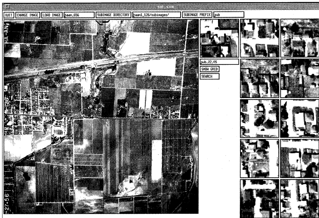
Figure 4. The image browsing tool for large aerial photos. The reduced-resolution version (left) of a large aerial photograph is searched for housing developments, which are then shown in thumbnail images (right).
